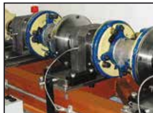
Full scale durability test of two wind generator couplings under extreme misalignment conditions.
