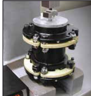
Coupling Axial Stiffness Test
