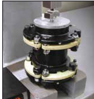
Coupling Axial Stiffness Test
