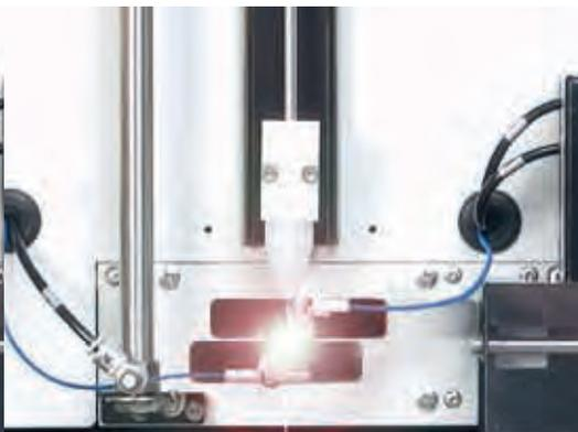
The wire is heated and expanded until it breaks.
