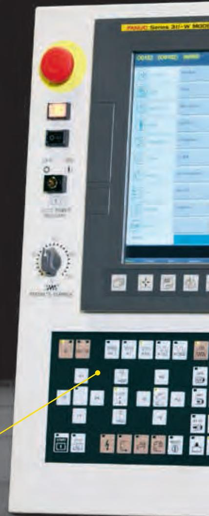
**15" colour display** with touchscreen for easy input of data with a minimum of keystrokes
