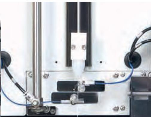
The guide roller retracts, the contact points are moved in to the wire.
