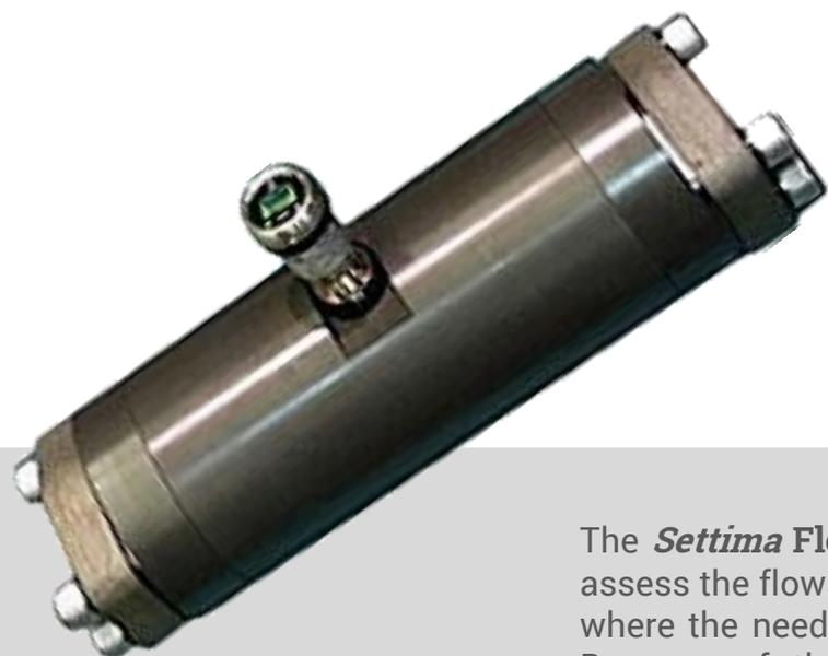
The **Settima Flowmeter** is an **extremely precise** instrument to accurately assess the flows of oils and fuels. It is installed on several pump test bench, where the need of a correct measure of flow is of paramount importance. Because of the volumetric functioning principle, the device is almost completely **independent of viscosity**. It can also operate and measure with both forward and reverse flow. The **Settima Flowmeter** is an excellent tool for **cost-sensitive applications**.
