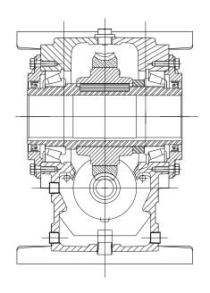
Hollow output shaft unit showing standard metric extension input shaft and American extension at the fan end.
