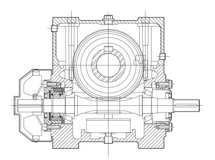
Underdriven unit with standard plug-in output shaft. Single and double extension shafts are available with metric American dimensions.
