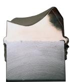
Section of electron beam welded wormwheel rim and centre showing the fusion of the bronze wormwheel rim onto the cast iron centre.
