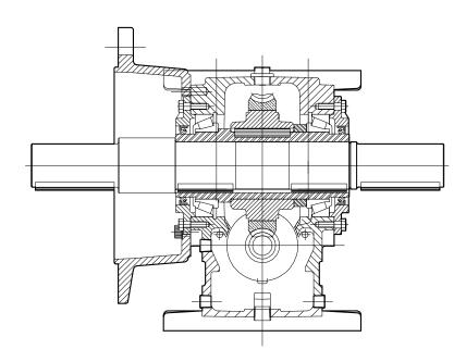
Dry well adaption fitted at the output of the WM Series unit. The non leak feature is particularly important on mixer applications in the food and chemical Industry.
