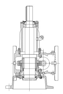
Agitator unit with output shaft up, particularly suited for cooling fan drives.
