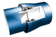
The junctions are made by inserting one pipe into the next. Watertightness is produced by compression of the elastomer joint gasket between two metal walls. The contact pressure on the elastomer joints increases as the internal pressure increases making the system highly reliable in operation.
