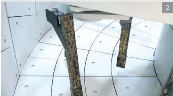
TEKA pan-type mixers THZ are also available with mechanical and hydraulic agitators. Mechanical agitators have a fixed rotation speed. The hydraulic agitators allow for infinitely variable rotation speeds.
