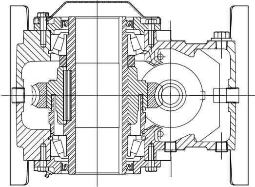
Dry well adaption fitted at the output of the WM Series unit. The non leak feature is particularly important on mixer applications in the food and chemical industry.
