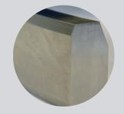
**The RTJ-Kamm gasket** combines the high pressure seal of an RTJ with the low stress sealing of a Kamm. The sealing faces are serrated and faced which means this style is ideal for use with damaged flange grooves or in low load applications.
