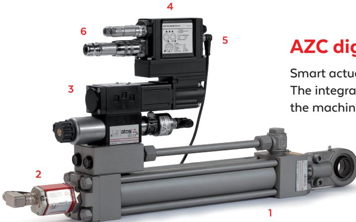
servocylinder 1 with position transducer 2, servoproportional valve 3, integral TEZ controller 4, connections to position transducer 5, to electric power, electronic signals and fieldbus 6
