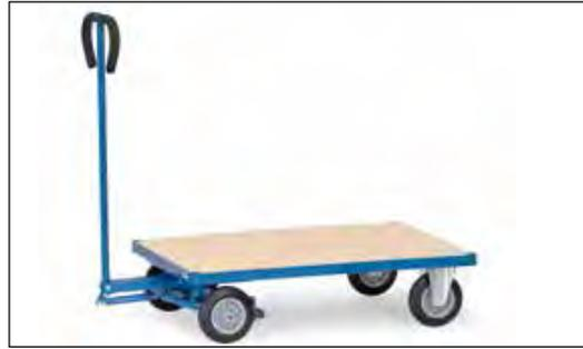
The add-on kit consists of an axle with 2 wheels, a bogie, a bracket and a drawbar with safety handle and automatic damped retraction in resting position. As well as an automatic wheel lock, according to the European Standard EN 1757-3 (safety of platform trolleys).
