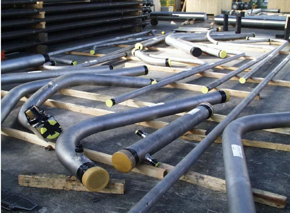
Picture 13: Pre-fabricated isometrics ready for transportation
