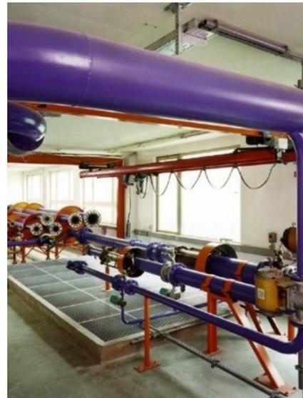
**Picture 15a/b: Control valve testing**
