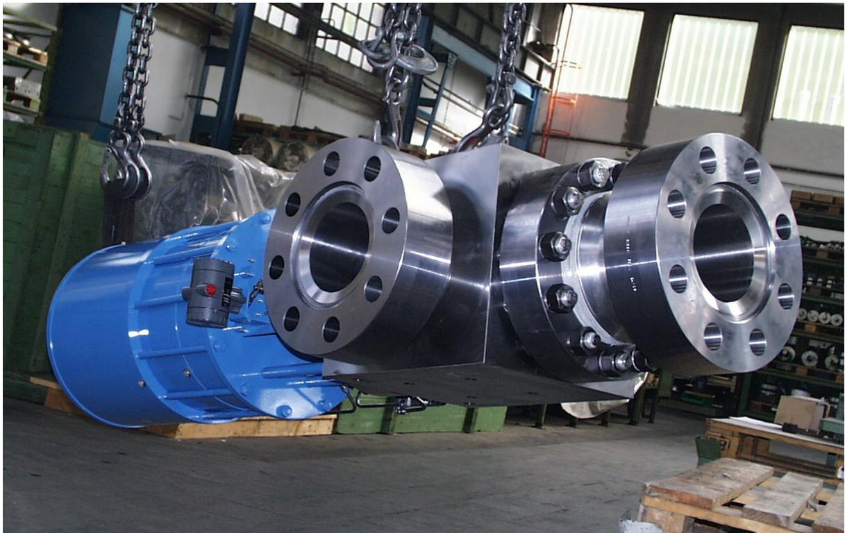
**Picture 7: A NS 10" Safurex<sup>®</sup> High Pressure Control Valve for the ABF urea plant in Malaysia**
