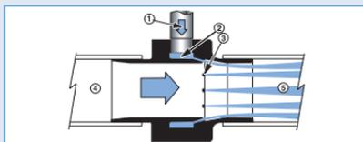
Compressed air flows through the inlet (1) into an annular plenum chamber (2). It is then injected into the throat through directed nozzles (3). These jets of air create a vacuum at the intake (4) which draws material in and accelerates it through the unit (5) for conveying over long vertical or horizontal distances.
