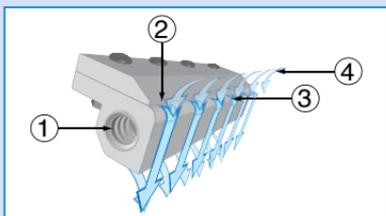
Compressed air flows through the inlet (1) into a plenum chamber. It is then throttled through a thin nozzle (2) extending the length of the Standard Air Knife. This primary airstream adheres to the coanda profile (3), which turns it 90° and directs the flow down the face of the unit. The primary stream immediately begins to entrain surrounding air (4), for an amplification ratio of 30:1 at 6" (152mm) away.
