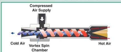
The Mini Cooler incorporates a vortex tube to convert a small amount of compressed air into two low pressure streams, one moving within the other in opposite directions (see page 143). The two airstreams exchange heat, producing cold air from one end of the tube and hot air from the other. A flexible hose directs the cold airstream at the surface to be cooled.
