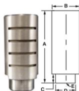
Heavy Duty Silencing Mufflers feature a corrosion-resistant aluminum outer shell with an internal stainless steel screen that protects valves and cylinders from contamination that could enter through the exhaust ports. This also keeps contaminants such as rust from being ejected at high speed from the exhaust port. The typical noise reduction is up to 14 dB.
