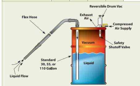
**Warning:** Do not use with any material with a low flash point or with flammable liquids such as fuel oil, alcohol, mineral spirits, gasoline, or kerosene.
