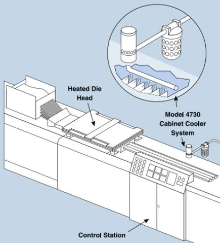
**The Problem:** In the pultrusion process, resin coated fibers are assembled by a forming guide, then drawn through a heated die. Residual heat from the die caused electronic malfunctions at the control station located immediately downstream.
