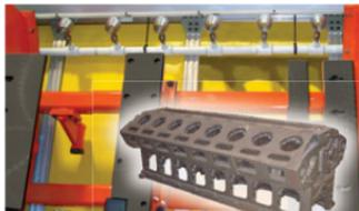
A series of Model 6042 Adjustable Air Amplifiers blows coolant off 16 cylinder diesel engines.
