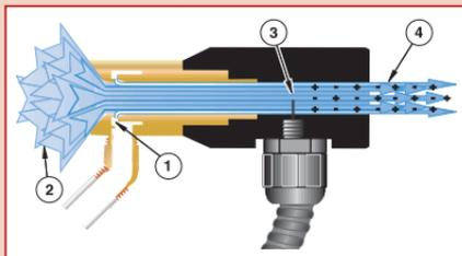
The Ion Air Gun incorporates a High Velocity Air Jet and electrically energized emitter point. A small amount of compressed air is injected into the air jet (1) inducing high volume flow of surrounding air (2) to pass through it.
