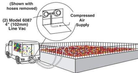
**Comment:** The compact design and simplicity of operation were the keys to success in this application. **The Line Vac also features large throat diameters for maximum throughput capability** - like the large plastic balls.
