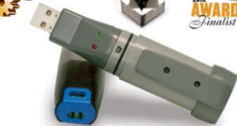
USB Data Logger for the Digital Flowmeter
