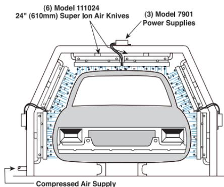
EXAIR's EFC (shown on page 4) is an electronic flow control for compressed air. It can sense when there is no car present and will automatically turn off the compressed air until the next car is moved into position. It is a perfect addition to this type of application.
