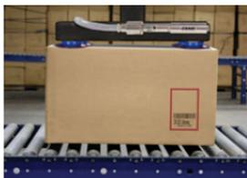
Compressed air use is minimized by selecting the exact vacuum level required to lift the heavy, porous cardboard cartons.
