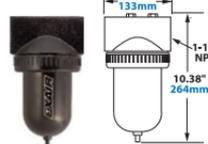
EXAIR's Filter Separators remove water, dirt and rust from your compressed air system. They prevent these contaminants from plugging or damaging the compressed air products. A Filter Separator should be installed prior to an oil removal filter, pressure regulator or valve.
