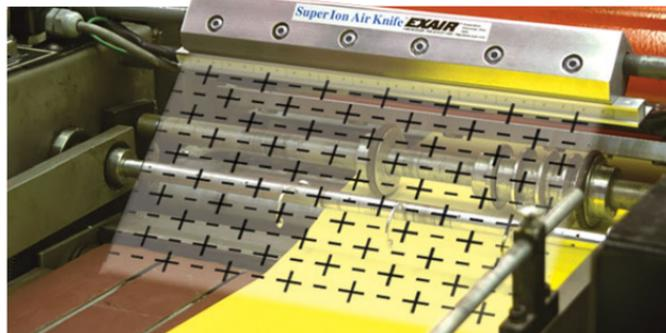
The Super Ion Air Knife eliminates static on a sheeter, so it picks up one sheet at a time.
