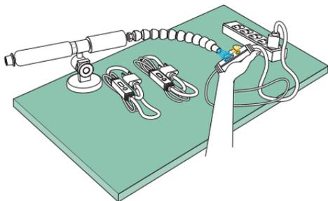
**The Problem:** A manufacturer of electrical heat tapes had a problem testing thermostats for accuracy. The heat tape is supposed to switch on when the outdoor temperature dips below 40°F to prevent pipes from freezing or ice from building up on a roof's edge. The liquid-tight thermostat of every tape had to be dipped into a bowl of ice water (thermometer checked at 36°F (2°C)) to make
