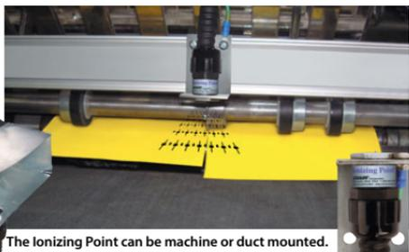
The Ionizing Point can be machine or duct mounted.
