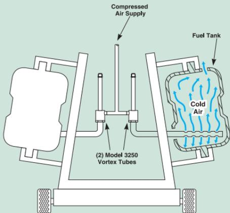
**The Problem:** Automobile fuel tanks are blow molded, then clamped to a fixture to prevent distortion during the cooling cycle. The cooling time of over 3 minutes required for each tank created a bottleneck in the production process.
