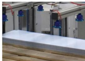
A series of bellows cups lift one plastic part at a time off of a pallet.
