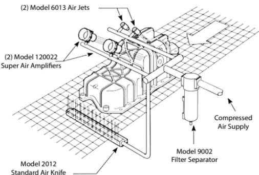
**The Problem:** A newly designed transmission pan presented a myriad of cleaning problems for the die-caster. Because the configuration included channels and blind holes as well as smooth surfaces, a “shaped” air pattern was required for proper cleaning. No single blowoff product would fit the need. An assortment of open copper tubes and drilled pipes was considered, but was rejected as too noisy and expensive
