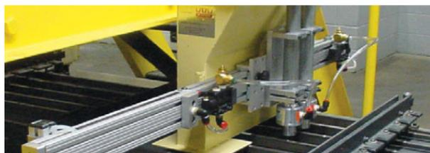
(2) Model 6083 1-1/2" (38mm) Line Vacs convey reject metal caps from a fluorescent lamp operation to a scrap bin.
