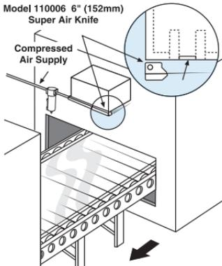
**The Problem:** Automotive glass is tempered by subjecting it to a series of heating and quenching operations. An infrared scanner maintains a uniform temperature across the glass surface by sending signals to a PLC that automatically
