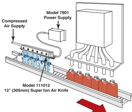
**The Problem:** A pharmaceutical company fills mouthwash bottles at a rate of 200 per minute. Friction with the conveyor belt and guide rails produced a static charge on the bottle surface that resulted in two problems. First, the static electricity sent false signals to an encoder responsible for monitoring material flow,
