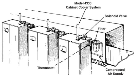
over the circuit breakers. Thermostat control assured that the **Cabinet Coolers would activate only when internal temperatures approached critical levels.** The panel doors were closed to prevent dirt infiltration and shock hazard. Downtime was eliminated.
