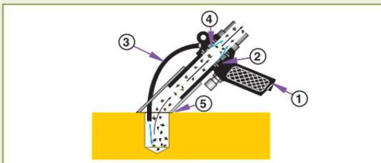
Compressed air, normally 80-100 PSIG (5.5 - 6.9 BAR), flows through the inlet (1) into an annular plenum chamber (2) when the trigger is depressed. A small amount of air is injected into the blow
