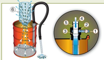
Compressed air, normally 80-100 PSIG (5.5 - 6.9 BAR), flows through the inlet (1) into an annular plenum chamber (2). It is then injected into the throat through directed nozzles (3). These jets of air create a vacuum at the intake (4) which draws material in, accelerates it through the unit (5), and directs it to the bottom of the drum. The airflow exhausts through the port in the drum lid. Airborne particles are trapped by the 0.1 micron filter bag (6).
