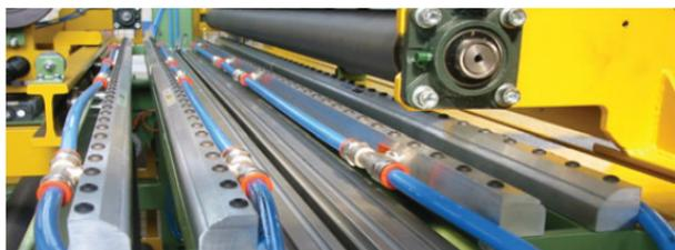
A series of Full-Flow Air Knives "float" layers of plastic film in this confined space of the machine.
