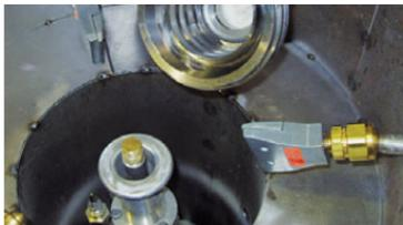
2" Super Air Nozzles blow off metal parts as they are lifted through a vacuum chamber.
