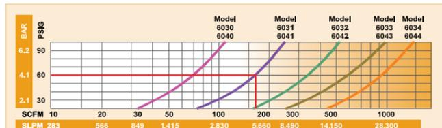
Total Output Flow with .002" (0.05mm) thick shim installed. Excludes downstream entrainment.
