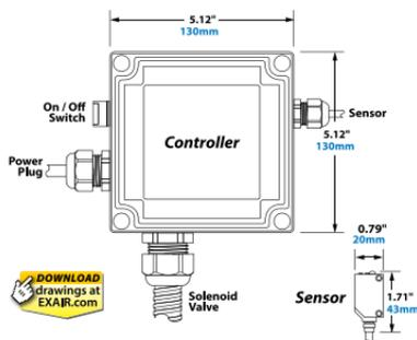
The timing control unit and the photoelectric sensor are equipped with a 9' (2.74m) power cord. The timing control unit is housed in a polycarbonate NEMA 4 / IP66 water tight enclosure.
