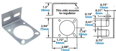
This optional mounting bracket fits Models 9008, 9033 and 9009 Pressure Regulators and includes the bracket and a locking ring.
