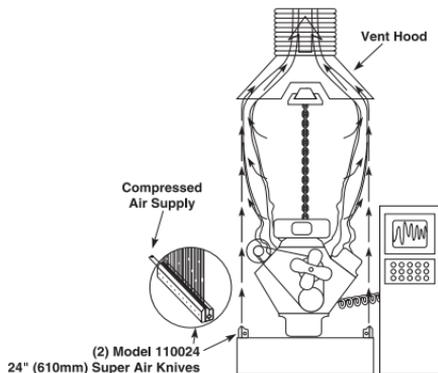
during the test, and the vent hood at the top of the stand had insufficient capacity to contain it.
