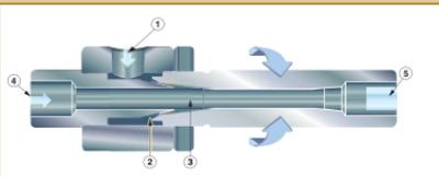
Compressed air flows through the inlet (1), then through an adjustable annular nozzle (2). As the airstream enters the vacuum flow, it expands and increases in velocity (3). A vacuum flow is induced, creating suction (4). The airflow that is drawn through the vacuum inlet mixes with the primary airstream, then exhausts on the opposite end (5).
