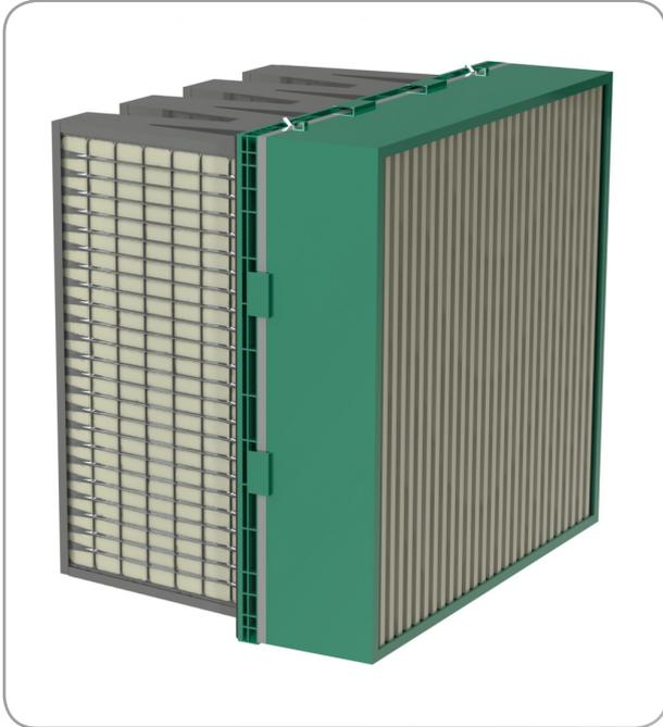
The Camfil CamClose is primarily used as a pre-filter to extend the service life of final filters by offering low initial pressure drop and high dust capacity. The filter is especially suitable for applications in humid conditions such as tropical and coastal installations, due to its downstream pleat separators and solid construction.
