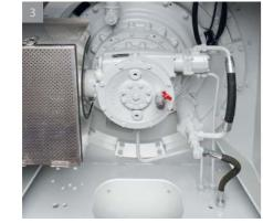
4 | Mixer sizes THZ 1125 G to THZ 6000 are driven by a foot-mounted motor which is connected to the gear box by a universaljoint cardan shaft. A hydraulic turbo-coupling or frequency converter for soft starts under load are also available. Flanged to the
