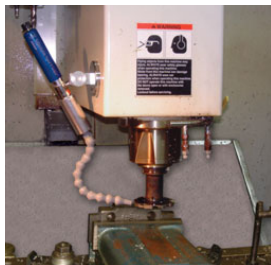
The Adjustable Spot Cooler replaces flood coolant and eliminates hours of cleanup on a cast iron machining operation.
