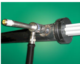
Cold air from a Model 3230 Vortex Tube quickly cools extruded plastic tubing.
