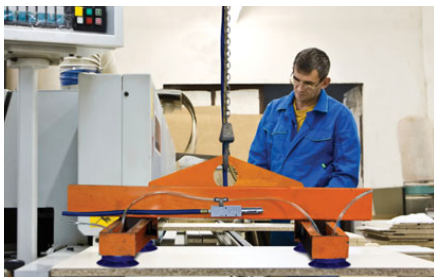
The Modular E-Vac, connected to a series of vacuum cups, lifts sheets of wood to a surface planer.
