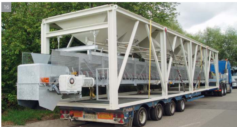
13 | TRANSMIX TDZ aggregate in-line silo plant TDZ 1500/3000 - R 4
