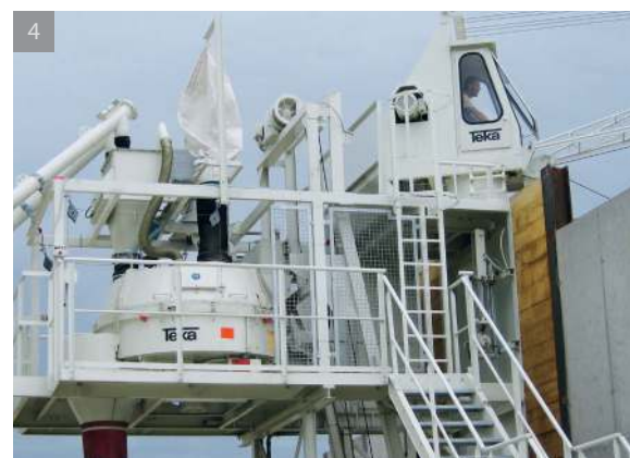
3 | TRANSMIX THZ 750 – S 4 scraper plant with manual scraper TS 12/13
