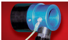
This special ionizer dries water based paint on car bodies and eliminates any static problems.
