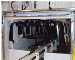
Bumpers, car bodies and fascia are cleaned of dust and fibers prior to painting.
