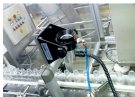
The Model 7292 Ion Air Cannon System eliminates the static and dust prior to filling the bottles.
