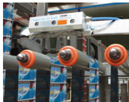
The Super Ion Air Knife eliminates the static charge on labels being applied to PET soft drink bottles.
