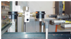
(2) Model 120022 2" (51mm) Super Air Amplifiers dry small parts as they move down along a parts conveyor.
