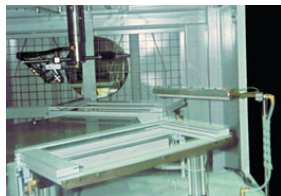
A Model 7212 12" (305mm) Standard Ion Air Knife System cleans metal frames prior to powder coating.
