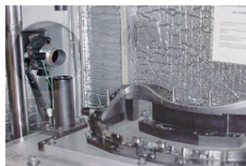
The Model 7292 Ion Air Cannon System eliminates static and dust from speedometer clusters prior to assembly.
