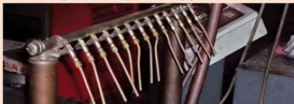
Turbulent compressed air blasts straight out of the pipe or tube. It not only wastes huge amounts of compressed air but also violates OSHA noise and dead ended pressure requirements.
