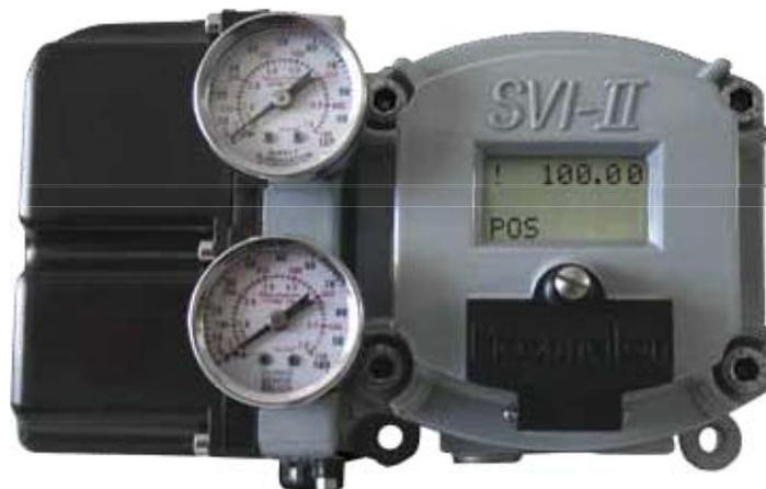
The GE Energy SVI II AP positioner with proven electronic and pneumatic technologies, combined with multiple sensors and smart software, offers high performance valve control with real-time diagnostics. The SVI II AP positioner is configured with a non-contact position sensor, a 32 bit ARM processor, a rugged I/P, and a poppet valve volume amplifier.
