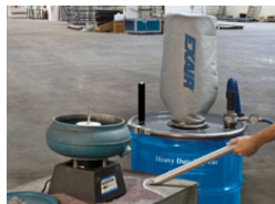
The Heavy Duty Dry Vac vacuums up abrasive garnet from the work surface surrounding a vibratory bowl used to deburr parts.
