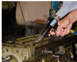
The Model 6194 Deep Hole Vac-u-Gun cleans the t-slots on a milling machine.
