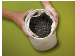
The 5 micron filter bag traps all the chips so no solids get pumped back out of the drum.
