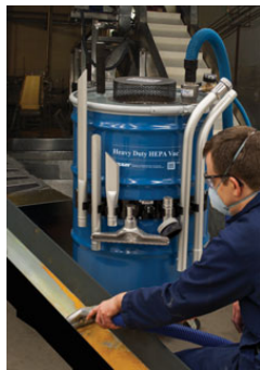
A technician uses a Heavy Duty HEPA Vac to perform scheduled maintenance on a pulverizer.
