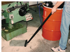
Room air remains dust free as the Chip Vac removes dusty absorbent.
