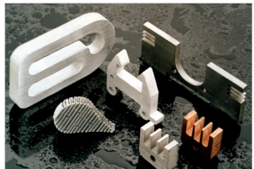
Technical parts, cut with an abrasive waterjet.
