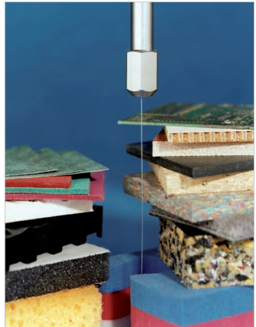
Various materials, cut with a pure waterjet.
