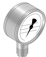
Connection at bottom
