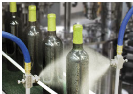
(2) Model EB1030SS atomizing nozzles are used to give a final sanitary rinse prior to labeling wine bottles.
