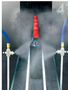
(2) Model EB1040SS nozzles are used to rinse wine bottles after capping.
