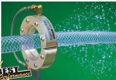
The Super Air Wipe uniformly dries a hose as it exits a bath.
