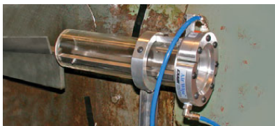
The Standard Air Wipe blows coolant off the part and back into the centerless grinder.
