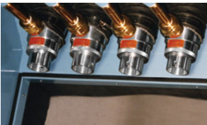
Adjustable Air Amplifiers are ducted to draw clean air for drying.
