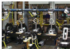
(5) Model 120022 2" (51mm) Super Air Amplifiers cool truck pistons.
