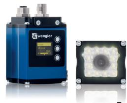
weQube and weQubeVision for digital image processing are equipped with five high-performance processors and an integrated image chip which make it possible to evaluate any number of predefined surfaces in a single step. In doing so, they compare the various colors within the respective surfaces. In this way, you can even check entire color sequences, e.g. for correct order - regardless of the object's orientation and position.
