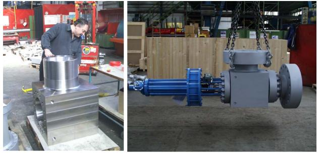
Picture 8A/B: The body (left) and complete NS 16" control valve for the Pardis Petrochemical Company in Iran made of 316L Urea Grade.
