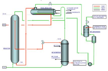
Figure 3: Stamicarbon's AVANCORE® Urea Process
