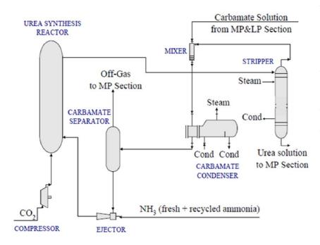
The figure on the left shows the Saipem urea high pressure synthesis section. Unique in this scheme are the horizontal kettle type high pressure carbamate condenser and the high pressure ammonia or self stripping which stripper, features already part of Saipem's urea technology for many decades.
