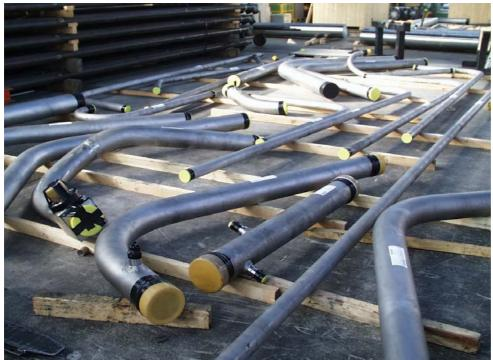
Picture 13: Pre-fabricated isometrics ready for transportation
