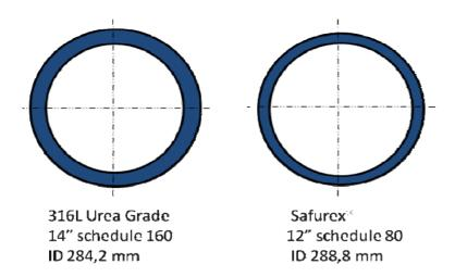
Figure 8: Safurex leads to downsizing of high pressure pipeline for lines of 12" and higher
