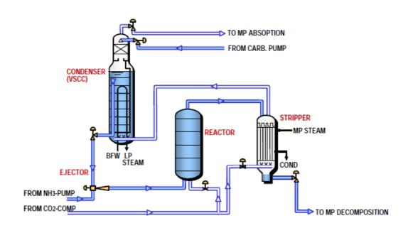
Figure 5: Flow scheme of the  $ACES21^{TM}$  High Pressure synthesis section
