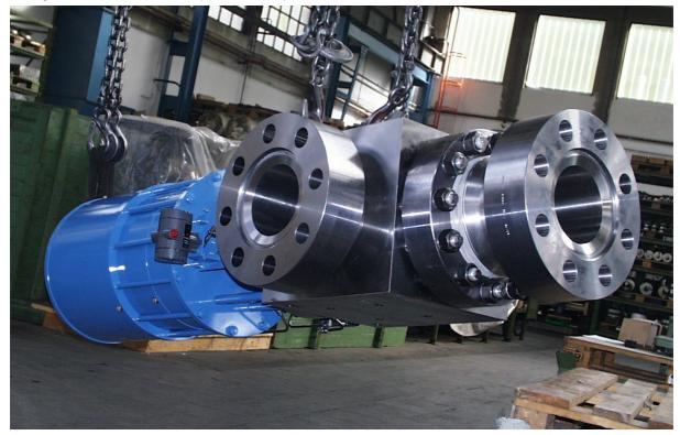
Picture 7: A NS 10" Safurex® High Pressure Control Valve for the ABF urea plant in Malaysia
