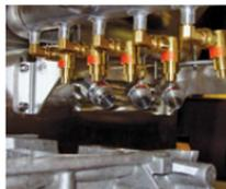
A combination of Model 6013 High Velocity Air Jets and Model 6042 Adjustable Air Amplifiers dry this engine casting.
