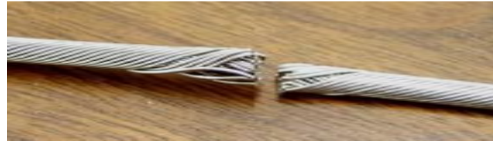
9"-6,500psi Valve Wireline Shear Test
