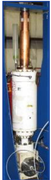
CH 55 on VG 300 valve prepped for PR2 testing in R&D environmental chamber
