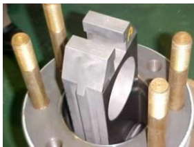
Diamond Lapped Seat Pockets, 2 micron Finish GE Aviation
