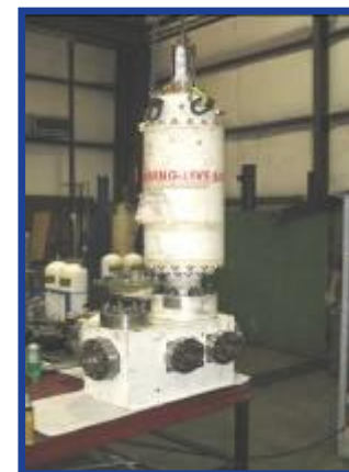
4" 5M Test Valve
