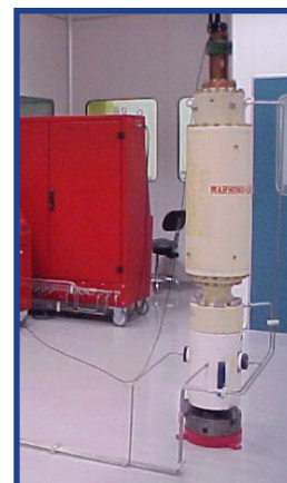
2" 5M Test Valve
