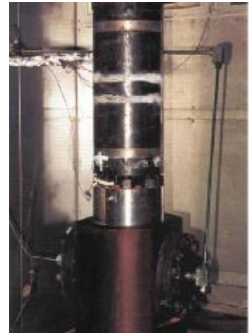
CH 55 on VG 300 valve prepped for PR2 testing in R&D environmental chamber
