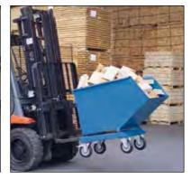
Sheet metal dump truck as waste bin with forklift truck.
