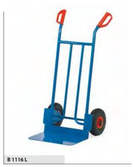
Handy tubular steel trucks with steel sheet blades, sturdy welded construction, blue RAL 5007. Safety grips. Steel sheet front shovel mountable, therefore exchangeable. Optionally solidrubber or pneumatic tyres on synthetic rims, hubs with roller bearings. Flat packed delivery.
