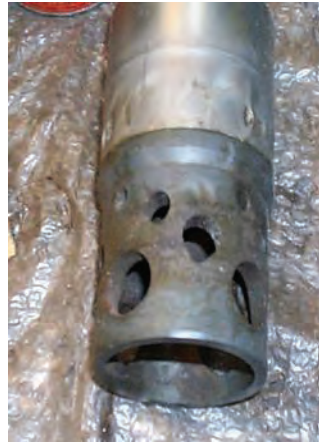
Figure 2: This choke trim has been used under similar circumstances, but in conjunction with a PRS device and shows minimal wear.
