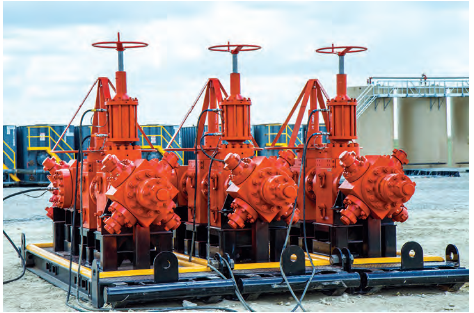
3-Well Frac Manifold
