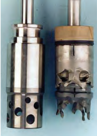
Figure 1: The choke trim on the left is a brand-new trim. The choke trim on the right is the result of a trim being used without a PRS device.
