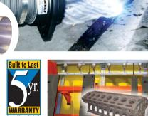
A series of Model 6042 Adjustable Air Amplifiers blows coolant off 16 cylinder diesel engines.
