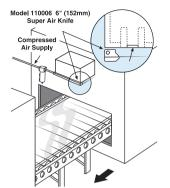
The Problem: Automotive glass is tempered by subjecting it to a series of heating and quenching operations. An infrared scanner maintains a uniform temperature across the glass surface by sending signals to a PLC that automatically
