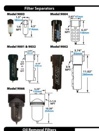
EXAIR's Filter Separators remove water, dirt and rust from your compressed air system. They prevent these contaminants from plugging or damaging the compressed air products. A Filter Separator should be installed prior to an oil removal filter, pressure regulator or valve.
