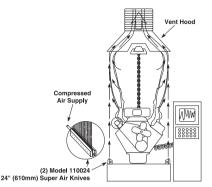
The Problem: The last step in an engine assembly process is "burn-in" on a test stand. Each engine is connected to a dynamometer and run for a period of one to five minutes. Residual machining oil on the head produced smoke
