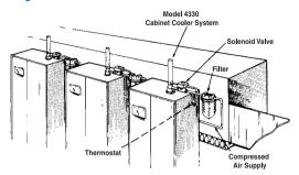
**Cooling Control Panels In A Glass Plant**
