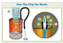
Compressed air, normally 80-100 PSIG (5.5 - 6.9 BAR), flows through the inlet (1) into an annular plenum chamber (2). It is then injected into the throat through directed nozzles (3). These jets of air create a vacuum at the intake (4) which draws material in, accelerates it through the unit (5), and directs it to the bottom of the drum. The airflow exhausts through the port in the drum lid. Airborne particles are trapped by the 0.1 micron filter bag (6).
