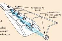
The Solution: They installed (5) Model 120022 2" (51mm) Super Air Amplifiers over the shakeout conveyor. The high output airflow from each Super Air Amplifier rapidly cooled the parts without shocking them (no cracks or imperfections from cooling too rapidly). When the part reached the end of the conveyor, the operator could proceed immediately. The backlog was completely eliminated.
