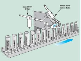
throughput. The vortex tube is the low cost solution for cooling parts, chambers, heat seals and various processes. They're easy to use, can be adjusted to produce cold air down to  $-50^{\circ}F$  (-46°C) and have no moving parts to wear out.
