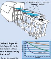
velocities. The uniform sheet of air from the Super Air Knife quietly swept the heat away within the first 2' (610mm) of the conveyor. Low air consumption and the compact size of the Super Air Knife were an added bonus.
