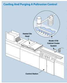
The Problem: In the pultrusion process, resin coated fibers are assembled by a forming guide, then drawn through a heated die. Residual heat from the die caused electronic malfunctions at the control station located immediately downstream.
