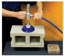
The vacuum level of the Adjustable E-Vac can quickly be changed from lifting lightweight payers to heavy cement blocks.
