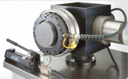
Extraction of the withdrawal sleeve with a hydraulic nut
